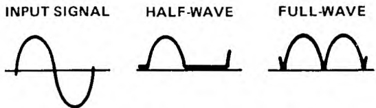
Figure 44. Rectifier Output-Voltage Waveforms
